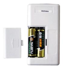
Figure 4. Batteries installation
